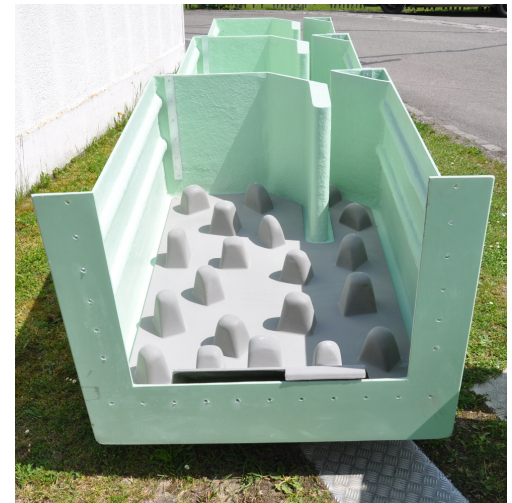
Figure 5: Stone imitations in prototype number two
