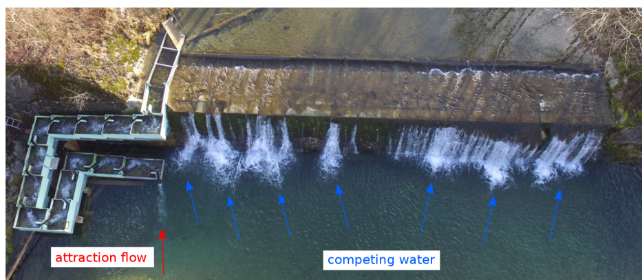
Figure 36: Steffstep on 30.01.16 with a medium discharge of 4.2 m 3 /s
